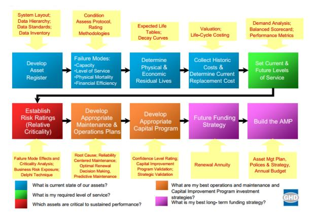
Figure 3: 10 Steps process to reach stormwater asset management program (City of San Diego, 2013)
