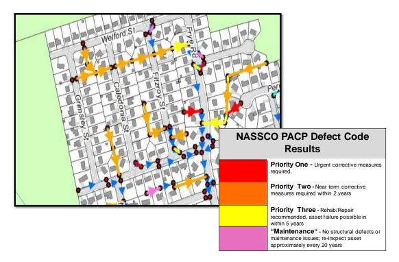
Figure 8: Example of Spatial Distribution of Priority Pipes (based on NASSCO PACP "QuickScore" (Eyre, Fortin, 2014)
